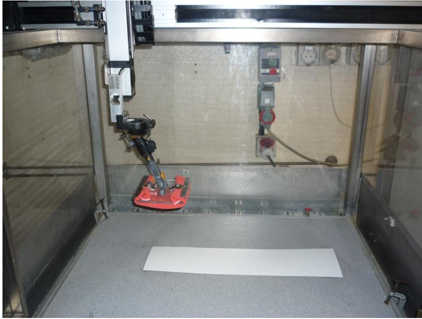
Figure 2: The automated cleaning rig fitted with a micro fibre cloth and placed furniture laminate surface.
