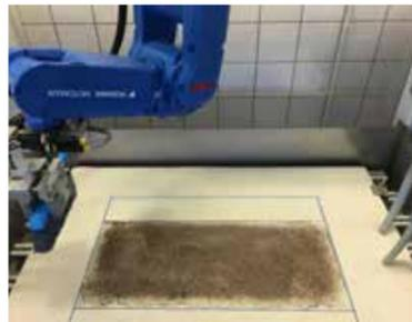
Figure 2. Robotic cleaning rig (Vikan, Denmark).
