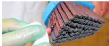
Figure 4a. Brush contamination using Brownes test soil.
