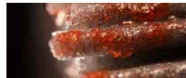
Figure 6b. Metal detectable bristles after cleaning (160x magnification).
